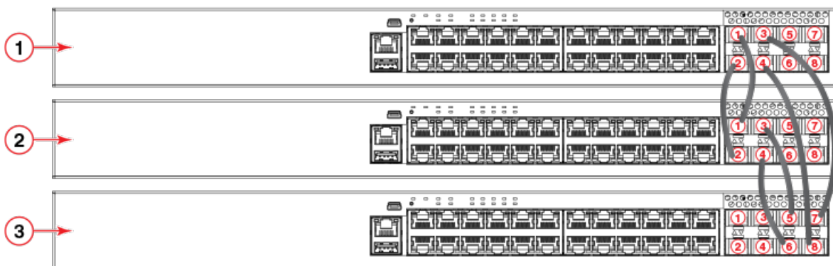
FIGURE 42 Ring stacking topology
